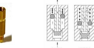
Pressurized discharge Pressurized deposited
